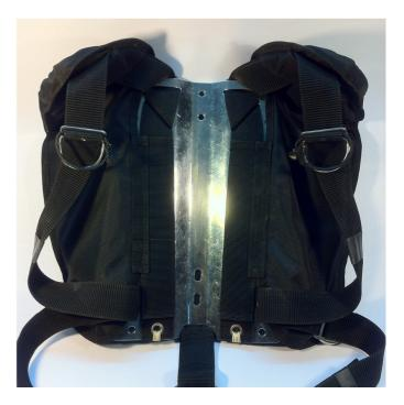
9 – Final adjustments of side to side position and height will have to be determined during actual dives. The picture shows a good starting point. If the back plate is worn low on your back you may have to move the counter lungs higher on the back plate. When the harness and counter lung height is properly adjusted the T-piece port will sit slightly behind the top of your shoulder.
