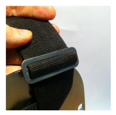
6 – The slide should sit close the top edge of your back plate. Check that the mounting strap is tight when you pull the harness upwards like when wearing the back plate. The strap needs to be tight to prevent side to side movement of the counter lung.
