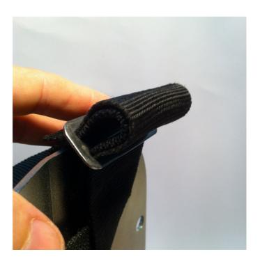
5 – The pictured loop of the harness makes it easier to get the strap though the second slot. Once the mounting strap is through both slots of the 3-bar slide, move the slide downwards.
